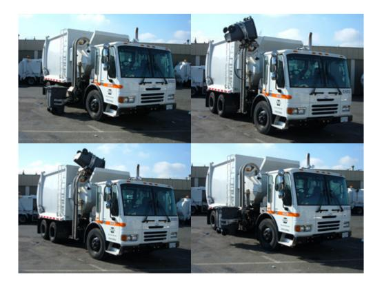
The continuous pack and decreased lifting cycle time means these trucks provide a substantial increase in system capacity over the original system. The other impact with these operating systems is because of the smaller range, and the smaller load dumping capacity (300 gallon versus 600 gallon loads) there is less strain on the lifting system, meaning lower cost of maintenance.
